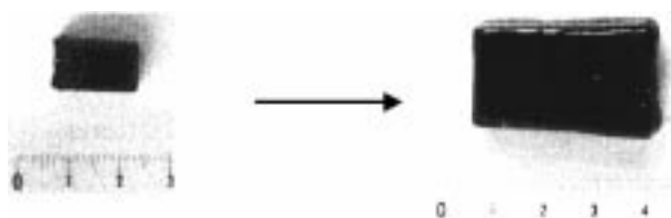
Figure 4. A hybrid 2% POM ferrogel a) after synthesis; b) swelled in an aqueous solution during four days (5.5 vol% \gamma\text{-Fe}_2\text{O}_3 particles).
